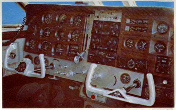
MARK 22 FRONT OFFICE. Here you'll find instrumentation planned to professional pilot standards. Flight instruments are "T" grouped directly in front of the pilot. Plex-ring lighting is ideal for night flying. PC release button and electric pitch trim and roll trim are integrated in the yoke. Overhead console gives convenient access to master switch and electrical control switches. Fuel selector and cabin pressurization controls are pedestal-mounted for easy accessibility.
