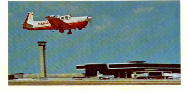
MARK 22 PRESSURIZATION . . . An AiResearch compressor provides both supercharging and pressurization for the MARK 22. The entire passenger area, baggage compartment and radio equipment racks are located *inside* the pressurized cabin. Cabin is pressurized to 4.0 psi. Cabin altitude at 20,000 feet is only 8,200 feet. Pressurization eliminates the need for cumbersome and uncomfortable oxygen masks.
